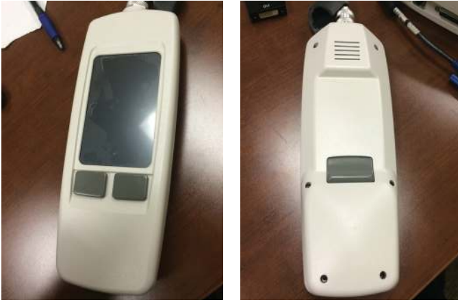
Figure 1: Existing pendant design was too large for a handheld device
