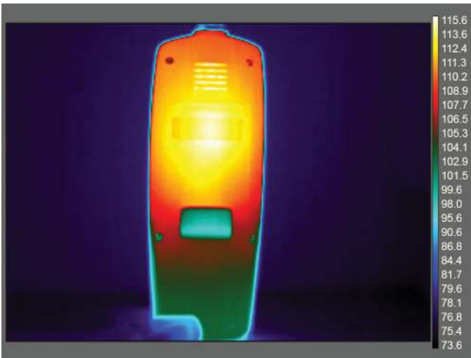
Figure 2: Thermal images of existing pendant design show that the pendant's surface temperature reached 125°F while operating at room temperature
