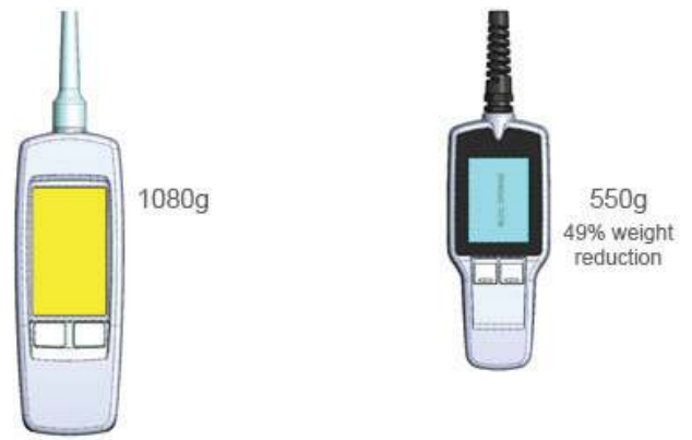
Figure 7: Before (left) and after (right) images showing the size and corresponding weight reduction
