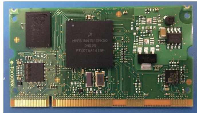
Figure 4: COM used to reduce size and power consumption of pendant
