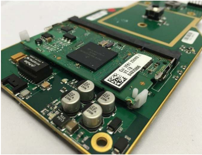
Figure 5: COM integrated into Synchroness-designed board
