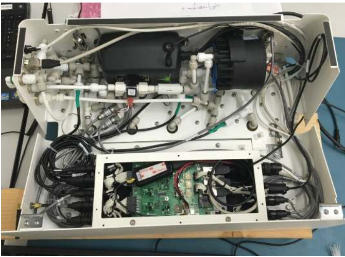
Figure 3: Prototype System during development shows hydraulic and electronics routing
